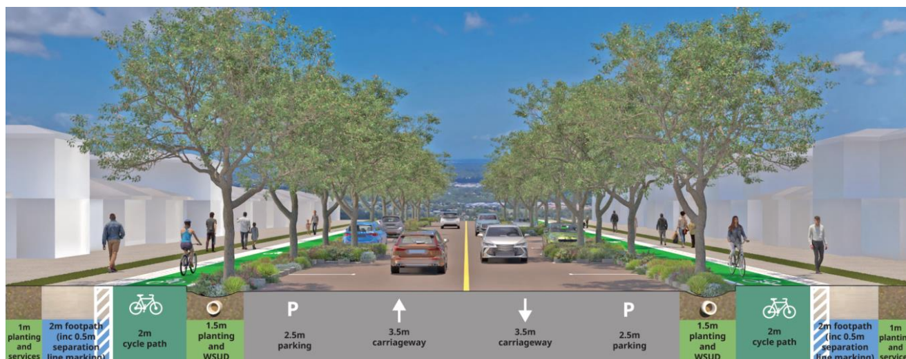
Figure 6: Cross section – District Collector (2 Lanes)
