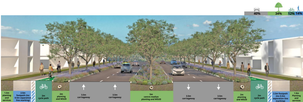
Figure 5: Cross section - 4 lane sub-arterial / arterial
