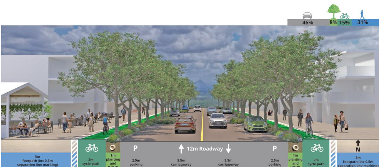
Figure 6: Cross section - Waraba Town Centre Main Street
