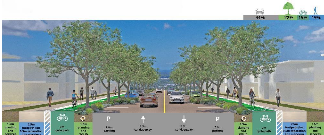
Figure 3: Cross section – 2 lane district collector
